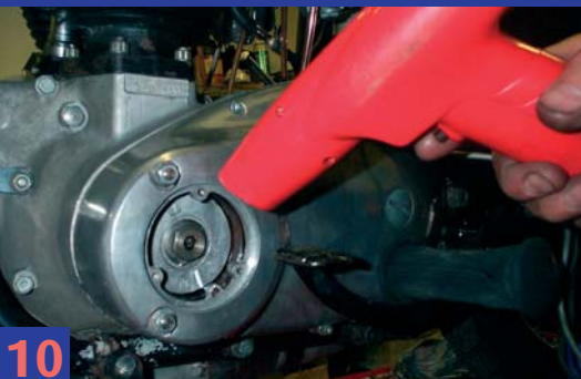
10 USING A STROBE LIGHT REV THE ENGINE TO 5000 RPM (THE IGNITIONS FULL ADVANCE SETTING 13 DEGREES) TURN THE STATOR PLATE ON ITS SLOTS UNTIL THE TIMING MARK ON THE ALTERNATOR ROTOR ALIGNS WITH THE POINTER ON THE CASE. ( USING A WHITE MARKER LINE ON THE ROTOR TIMING MARK WILL HELP).
