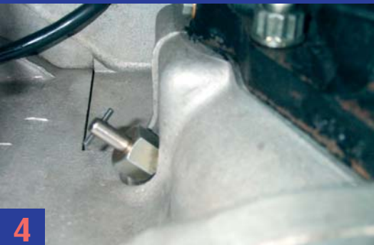
4 SET THE CRANK SHAFT IN THE STATIC B.T.D.C POSITION. THIS WILL VARY WITH DIFFERENT MODELS OF MOTORCYCLE SEE YOUR MANUAL FOR SPEC.
